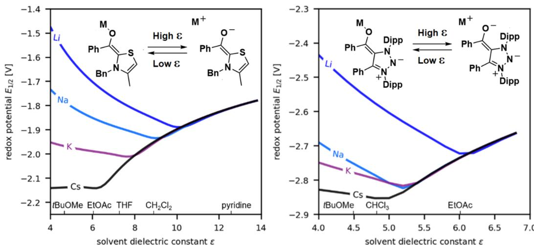
**Figure 6.** Influence of the cation (Li, N, K, Cs) on the first reduction potential of  $\text{BI}^{-}\text{M}^{+}$  salts derived from carbenes 1 (left) and 3 (right) with the solvent polarity.
