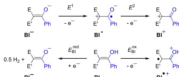
Figure 3. First and second oxidation of BI<sup>-</sup> (top); reduction and oxidation of BI (bottom).
